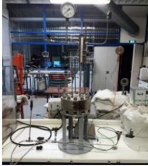
Gaseous H 2 permeation setup
