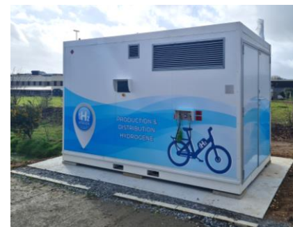
Production H2: 1Nm 3 /h Distribution: 300bar
