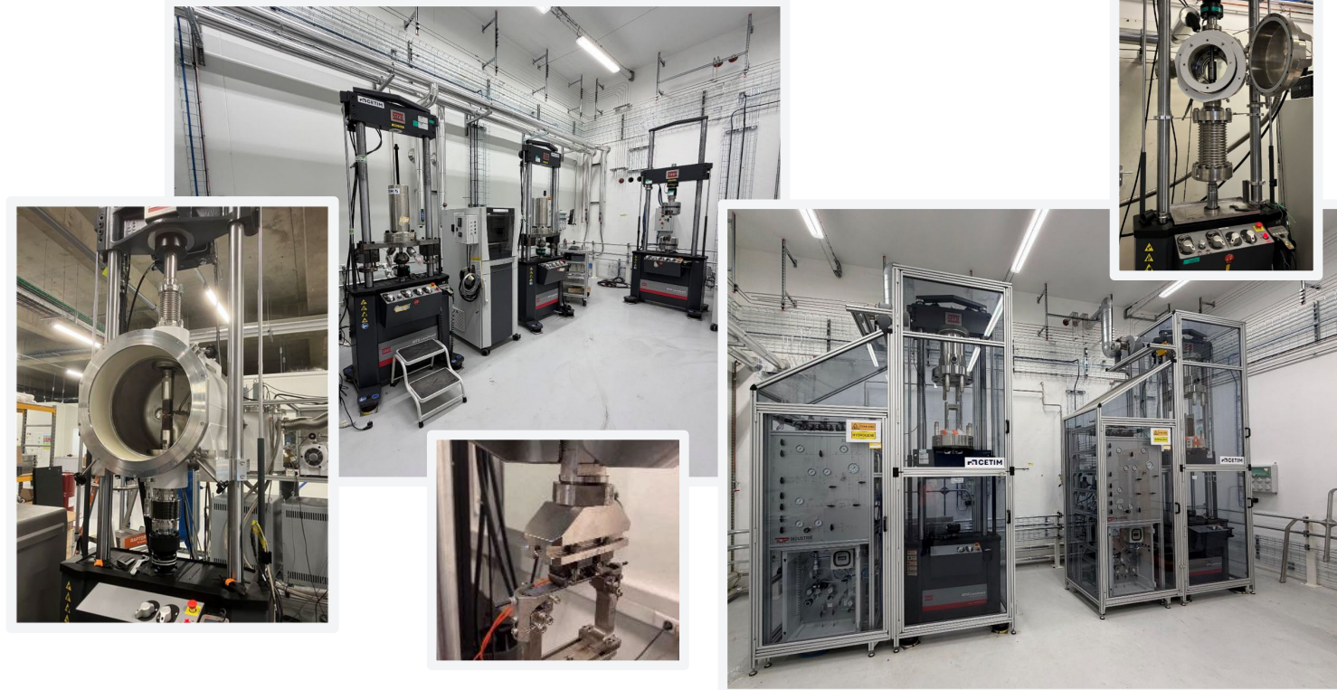
Mechanical environmental machines operating in a wide pressure (up to 400 bar) and temperature range (-253°C to 450°C) for multi-materials expertise
