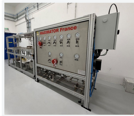
H 2 rapid gas decompression: 1000 bar & 70 bar/min
