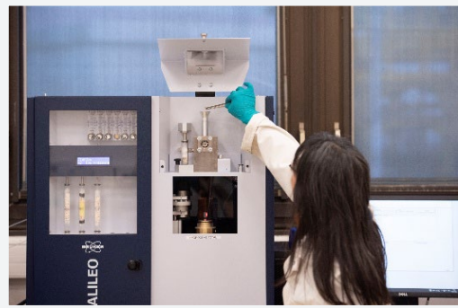
H 2 quantification: Thermo-Desorption Spectroscopy
