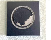
Blistering and detachment of thin oxide coating on 316L substrate
