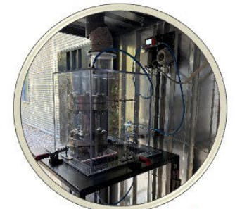
Cyclic pressurization 10 to 100 bars
